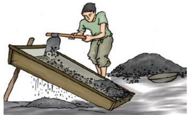
Fig. 5.7 Pebbles and stones are removed from sand by sieving
