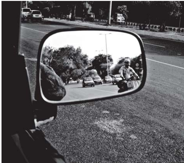
Fig. 15.20 Convex mirror as side view mirror
