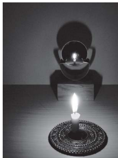
Fig. 15.19 Image formed by a convex mirror
