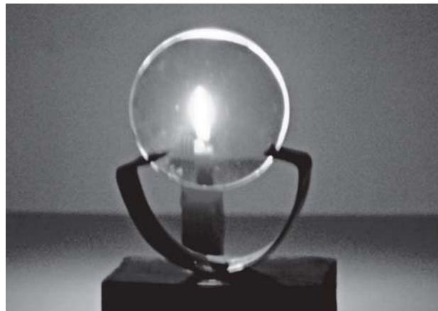
Fig. 15.27 Image formed by a concave lens
