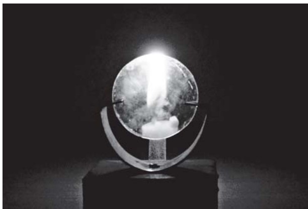
Fig. 15.26 Virtual image formed by the convex lens
