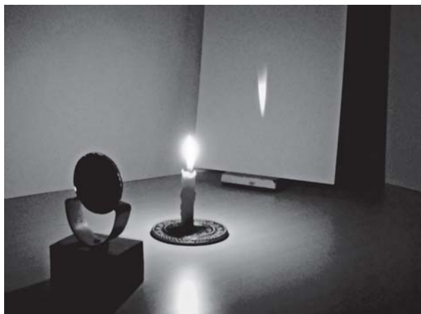
Fig. 15.15 Real images formed by a concave mirror
