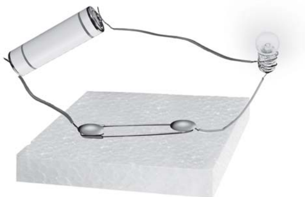
Fig. 14.7 An electric circuit
