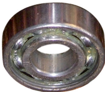
Fig. 12.16 : Ball bearings reduce friction
