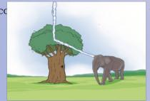
TOUCH POTENTIAL: If one part of a tall animal's body is in contact with the ground while another part, at a higher elevation, comes in contact with a lightning-struck object, a partial current may pass through its body
