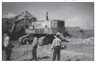
Fig. 12.2 : Noise monitoring at Panchpatmalai Bauxite Mine
