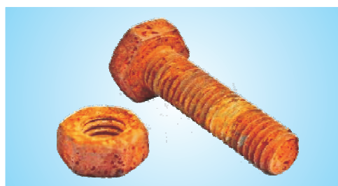
Fig. 4.9: Rusted nuts and bolts of iron
