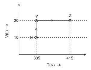
Considering only P-V work is involved, the total change in enthalpy (in Joule) for the transformation of state in the sequence  $X \to Y \to Z$  is \_\_\_\_\_.
